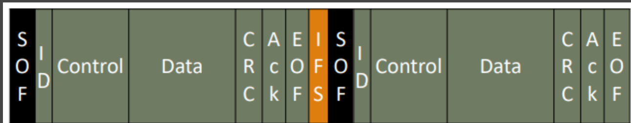
Figure 2: CAN frame fields of two back-to-back frames.
